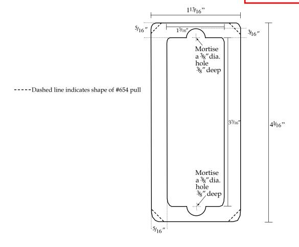
Mortise  $3^{7/16}$ " long x  $1^{3/16}$ " wide x  $^{3/8}$ " deep. Use brads provided to attach pull to door through the holes at both ends inside the recess.
